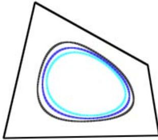
**Figure 13:** An example of spline curves of degrees 2, 3, and 4 where the inscribing curves have been scaled by 0.7 about a centre of the control polygon computed as the average of the control points.
