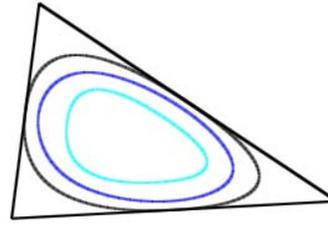
**Figure 11:** An example of spline curves of degrees 2, 3, and 4.
