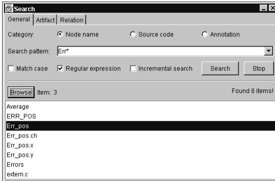
Figure 4: General search. Search for nodes whose names match the regular expression of Err* .
