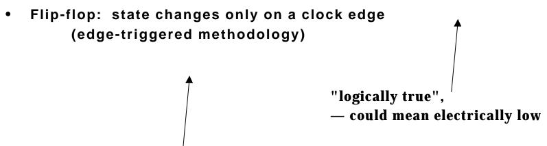
A clocking methodology defines when signals can be read and written — wouldn't want to read a signal at the same time it was being written
