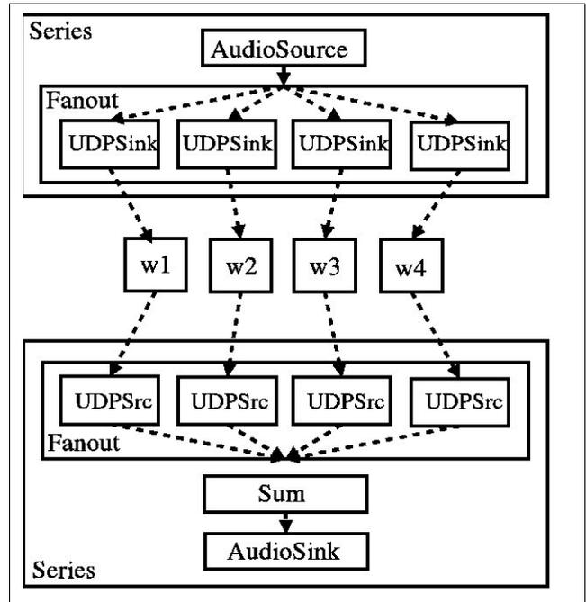
Figure 8. Real-time distributed harmonizer
