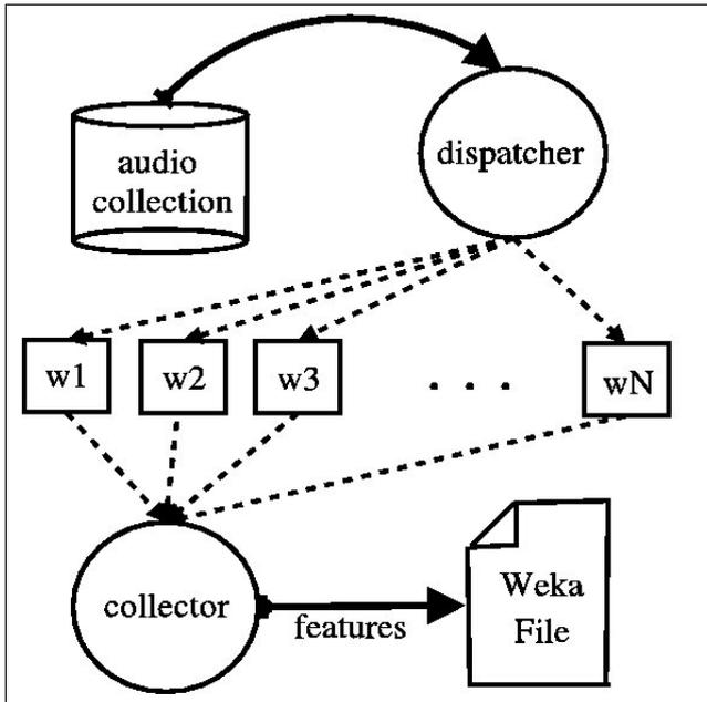
Figure 7. Distributed audio feature extraction
