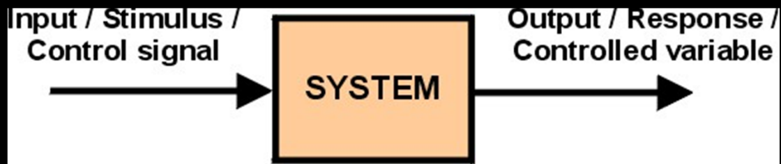
Fig.14 Open loop control system
