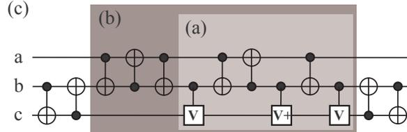
Figure 9: Optimal circuits for (a)  $(a, b, c) \mapsto (b, a, c \oplus ab)$ , (b)  $TOF(a, b; c)$ , and (c)  $TOF(a, c; b)$ .
