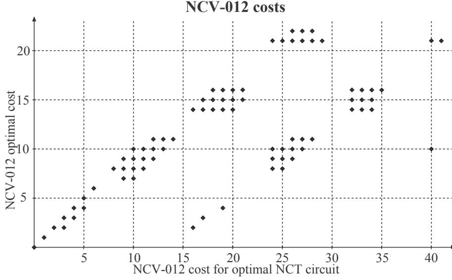
Figure 6: Optimal NCT (X-coordinate) vs. optimal NCV-012 (Y-coordinate) circuits for the NCV-012 cost metric. Each data point corresponds to a number of functions.
