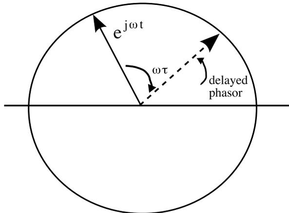
Figure 1: The effect of delaying a phasor by  $\tau$  sec. The dashed phasor is the delayed version of the original
